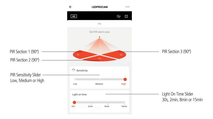
Notice the PIR detection can be combined to allow for a full 270° area of detection or as low as a 90° area of detection from the left, right or centre. You can also enable or disbale the PIR detection areas to suit your installation environment i.e. left and right areas to detect only while the central area remains disabled.
